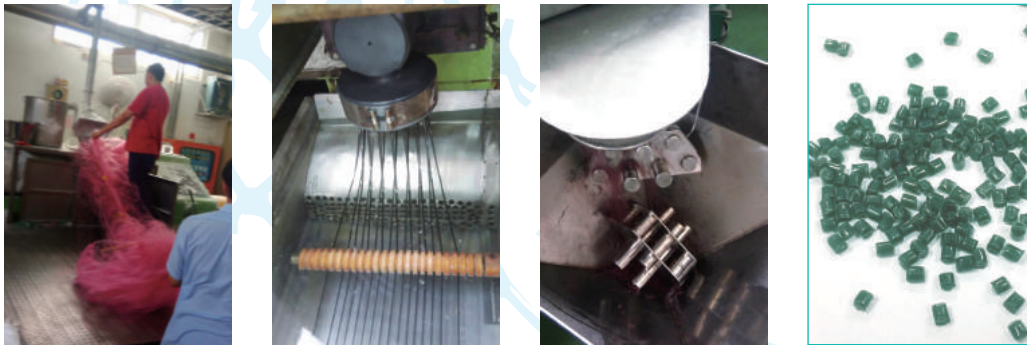
FISHING NETS VIA MELTING, DROWING AND CUTTING INTO CHIPS
